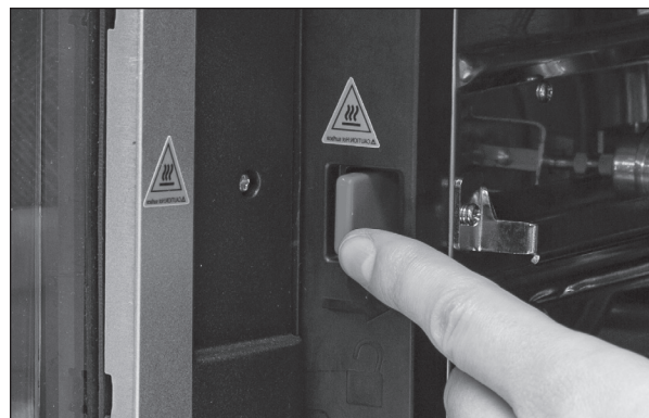
FIG. H: Hold switch in left position to insert/remove Round Basket
